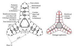
Fig.33: Burj Khalifa plan and structural axonometric <u>Thehexagonal central core</u> consists of reinforced concrete shear walls with thicknesses varying between 130cm at the bottom to 50cm at the top (below the spire) through the height of the building
