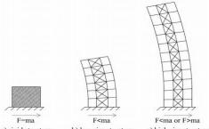
Fig?: The behaviour of a building during an earthquake **2.3 The Structural system of Tall Buildings.**
