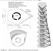
Fig45: HSB Turning Torso plans and structural axonometric.
