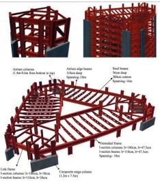
FIGURE 4.39 Commerzbank Tower structural axonometrics
