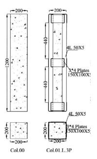
Figure 5. The geometry of the tested columns. (Belal, et al., 2014)
