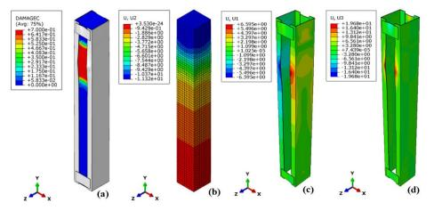
Figure 9. The damage of column 1-2Pls and the displacements in the column and the steel cage.
