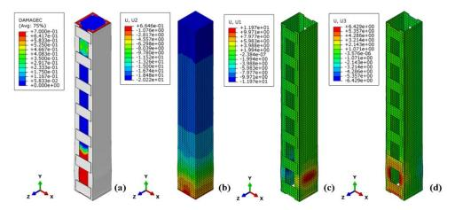
Figure 12. The damage of column 4-7Pls and the displacements in the column and the steel cage.
