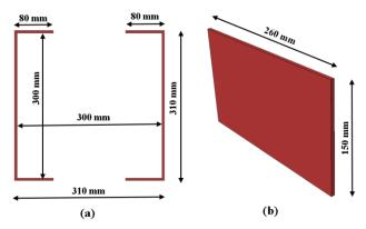
Figure 2. (a) Details of the two C-channels steel cage; (b) The connecting Batten plate.
