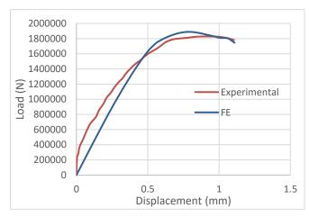
Figure 7. The load-displacement curve of the experimental and FE model of the second column.
