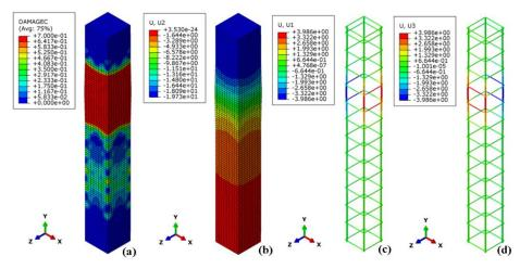
Figure 8. The damage of the reference column and the displacements in the column and the reinforcement steel.
