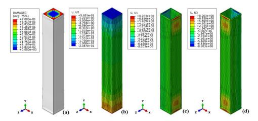
Figure 14. The damage of column 6-1Pl-In and the displacements in the column and the steel cage.
