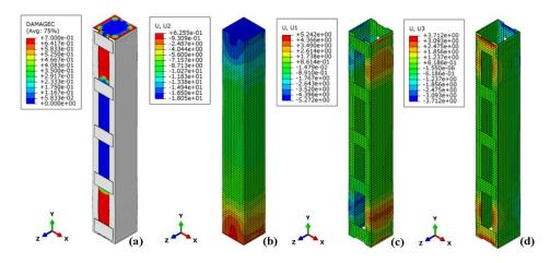
Figure 11. The damage of column 3-5Pls and the displacements in the column and the steel cage.
