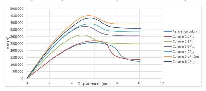
Figure 15. The load-displacement curve for all columns.
