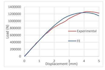
Figure 6. The load-displacement curve of the experimental and FE model of the first column.
