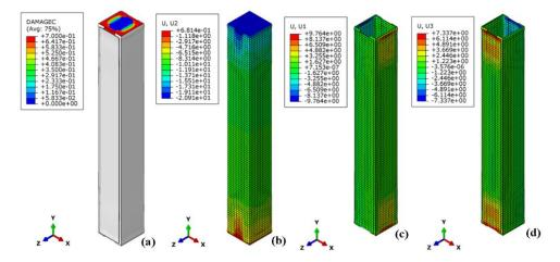
Figure 13. The damage of column 5-1Pl-Out and the displacements in the column and the steel cage.
