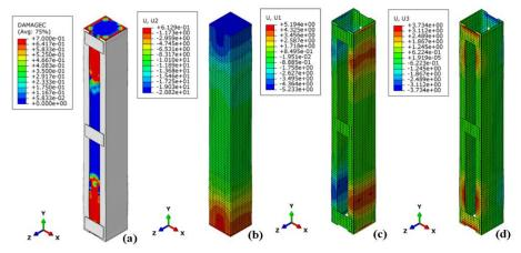
Figure 10. The damage of column 2-3Pls and the displacements in the column and the steel cage.
