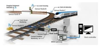
Fig.1: remote condition monitoring of the rail system [9].
