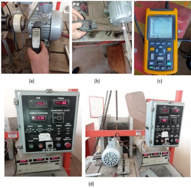
Figure 9. Testing instruments for the electrical motor where (a) Infrared Thermometer (b) Tachometer (c) Digital multimeters (d) Power Analyzer
