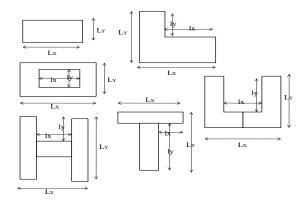
Figure 2. Different Plan Shapes
